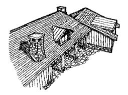
B. Major roofs within the Open Sage and Sage/Shrub Areas are limited to a maximum 8:12 pitch (with 6:12 preferred), while minor roofs on dormers and porches may be as low as 3:12 pitch. Low-pitch roofs should be covered with appropriate materials for the low slope, such as metal.
